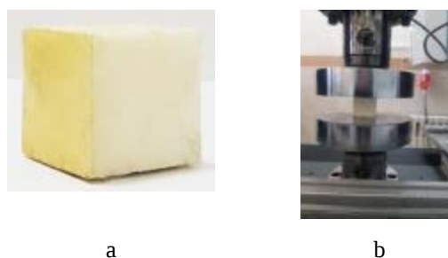
Figure 3: (a) a polyurethane foam sample, (b) compression testing machine.
